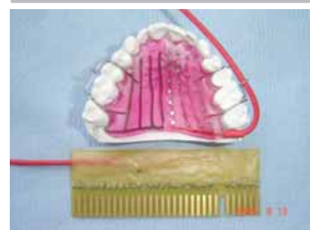
Figure 9. The finished plate and circuit board.
