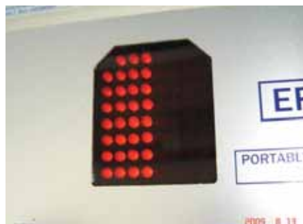
Figure 2. A modern control unit showing that the tongue is in contact with the left half of the palate during speech.
