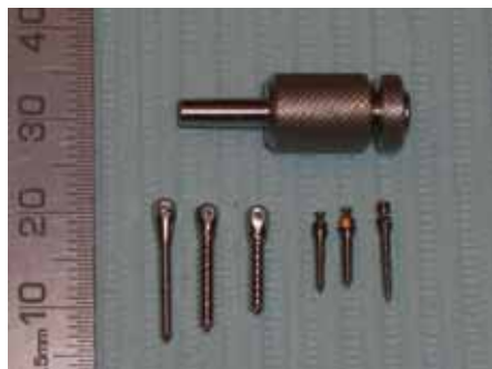
Figure 3. Variation in screw head design and size. Short screw driver (top); 1.5–2.0 mm diameter stainless steel in lengths of 8–12 mm with short and long head designs (left); 1.2 mm diameter Ti alloy in lengths of 6–8 mm with small head and bracket head designs (right).
